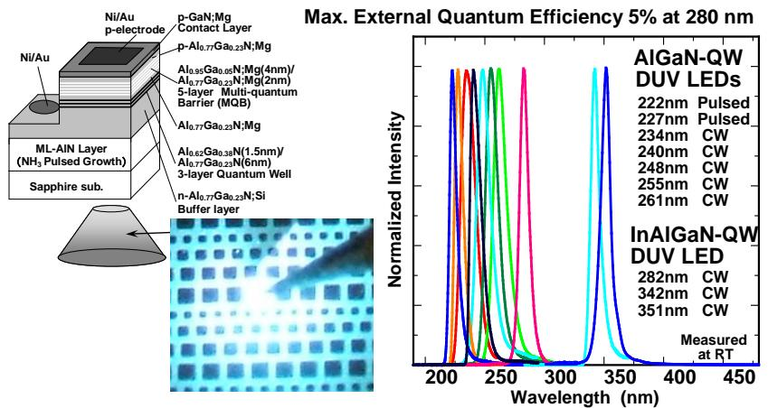
Fig. 3. Recent achievements of deep-UV LEDs using AlGaN-based semiconductors
