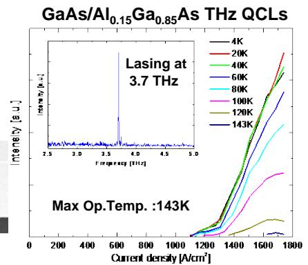
Fig. 4. Achievements of high-temperature operation of GaAs-based THz-QCLs
