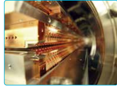
In-vacuum Undulator Stronger X-rays are generated by arranging magnets close together.
