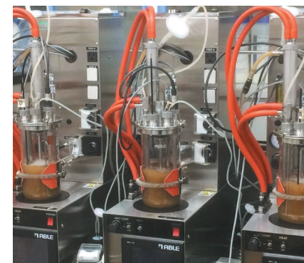
Genetically engineered E. coli used to produce maleic acid for industrial use @CSRS
