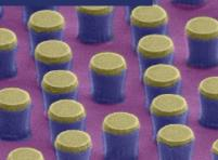
Silicon dioxide micropillars for quantum computing, 4 µm tall (blue) with 100 nm thick chromium metal caps (yellow). That's small!! @CEMS
