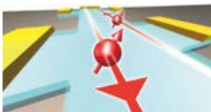
Schematic of the quantum Hall effect on the surface of a topological insulator
