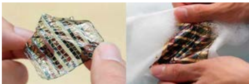
(Left) Ultraflexible organic solar cells manufactured on a 1 μm-thick plastic film. (Right) Photograph of the washing process for the devices conforming to a dress shirt.
