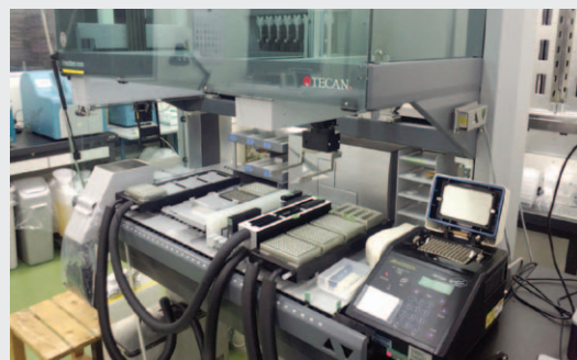
Figure 1: The automated CAGE cDNA preparation system for rapid genome-wide gene expression analysis.
