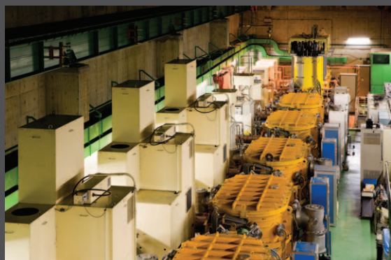
RILAC ion accelerator at the RIBF
