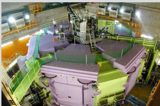
Superconducting Ring Cyclotron at the RIBF
