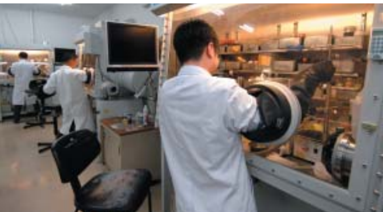
The six glove boxes are put to full use to explore the possibilities of the new catalysts.
