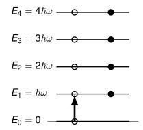
• The excitation energy from the ground state to the first excited bosonic state is  $\hbar\omega$
